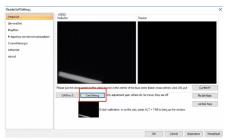
Just increase the value of Camera  $1 \rightarrow$  Sensor $\rightarrow$  Gain. Generally, the camera is 3 meters away from the projection imaging area, and the gain value is set to about 15-30.
