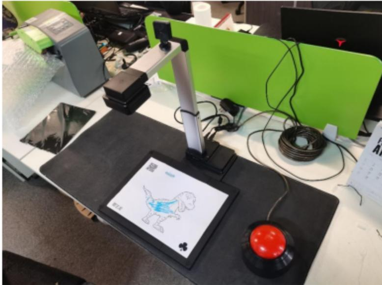
(2) The scanner usb must be connected to the computer rear usb3.0 port, 5V 1A power supply independently; button directly connected to the computer rear usb port.
