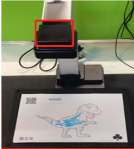
(4) The scanner must be placed in the middle of the black mat, and the scanner must be placed on the surface of the pure black mat. When you open the scanner, only game paper and black borders are displayed in the video source, with no other background colors appearing.
